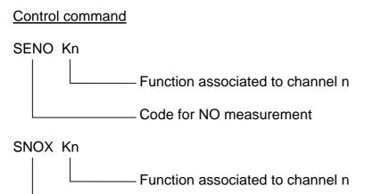
\_\_\_\_\_ Code for NO<sub>x</sub> measurement
